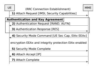
Figure 2: LTE Attach Procedure including the AKA.
